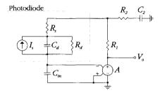
Fig. 2. Small-signal equivalent model of the PIF-circuit. The photodiode is represented by the photocurrent generator  $I_s$ , the capacitor  $C_d$ , and the resistors  $R_d$  and  $R_s$ . The input capacitance of the operational amplifier is represented by  $C_{in}$ .
