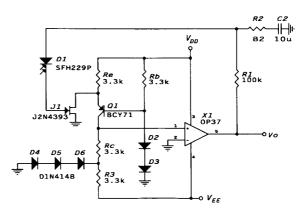
Fig. 4. Circuit diagram of the implemented PIF-circuit. Power supply decoupling components are not shown.
