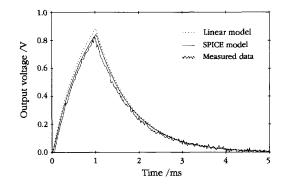
Fig. 5. Pulse response of the implemented PIF-circuit. The amplitude and width of the current pulse in the photodiode are 10 pA and 1 ms, respectively (measured and simulated data).
