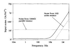
Fig. 7. Input noise of the SPICE model of the implemented PIF-circuit. Noise contributions from a small resistor in series with the photodiode and from a large resistor in parallel with the photodiode are also shown for comparison. Simulation results.
