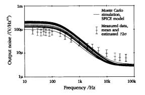
Fig. 8. Output noise of the implemented PIF-circuit. Measured and simulated data.
