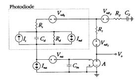
Fig. 3. Noise equivalent circuit of the PIF-circuit. The photodiode noise is represented by  $I_{nd}$  and  $V_{nR_s}$ , the amplifier noise is represented by  $I_{na}$  and  $V_{na}$ , and the noise in the feedback network is represented by  $V_{nR_1}$  and  $V_{nR_2}$ .
