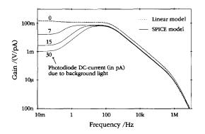
Fig. 6. Magnitudes of the transfer function of the implemented PIF-circuit. The pole given by  $\tau_d$  and the gain constant of the transfer function are dependent on the bias point of the photodiode. Simulation results.
