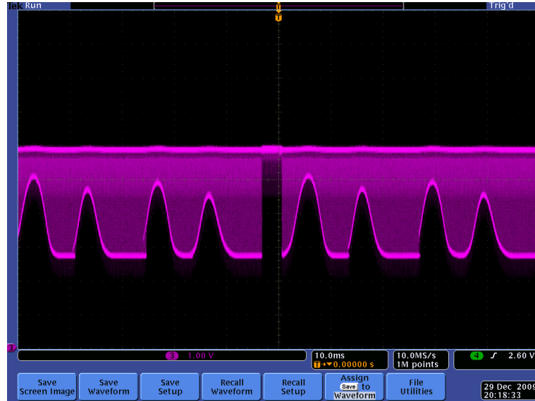
Fig. 4: One of the first measurements of the CCD output on an oscilloscope. On the screen, there are two consecutive readouts of CCD. The detector window was covered by four thin paper stripes. Note the end-of-register signal in the middle of the screen and the blooming which slightly overlaps the less illuminated areas.
